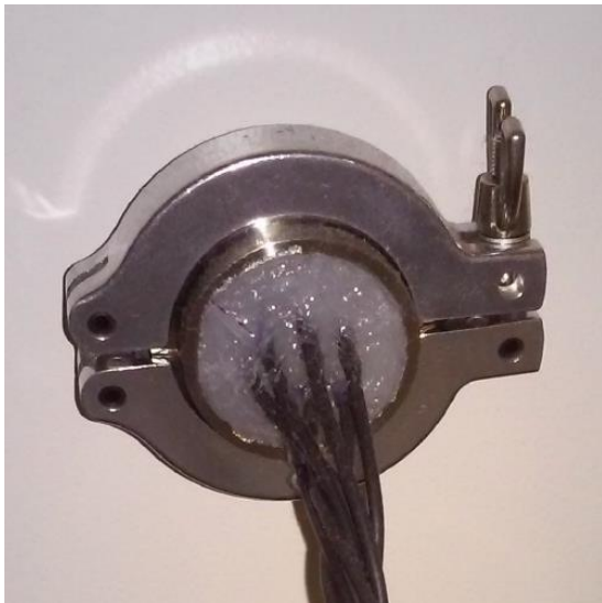
Figure 3-2. Cell Cable Glovebox Feedthrough
