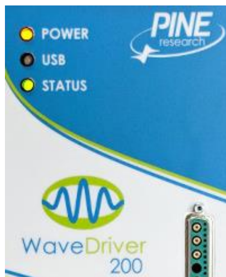
Figure 4-3. Indicator Lights on the Front Panel of the WaveDriver 200
