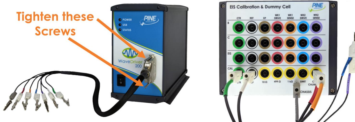
Figure 10-3. WaveDriver 200 Connections for Cell Cable Calibration
