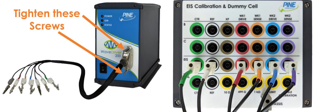
Figure 10-4. WaveDriver 200 Connections for a Simple EIS Test
