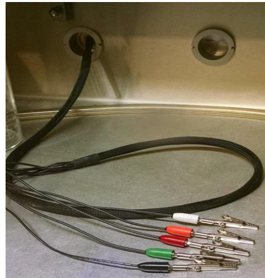
Figure 3-2. Cell Cable Glovebox Feedthrough
