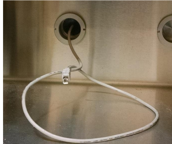
Figure 3-1. USB Cable Glovebox Feedthrough
