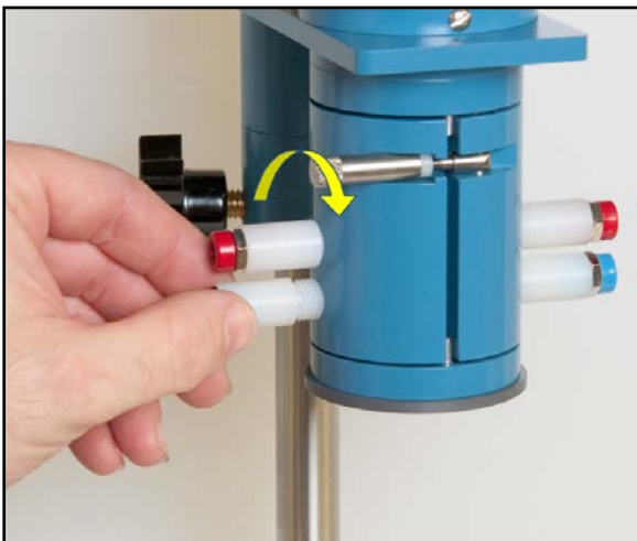
Figure 3-6. Insertion of Newly Replaced Brush Assembly.
