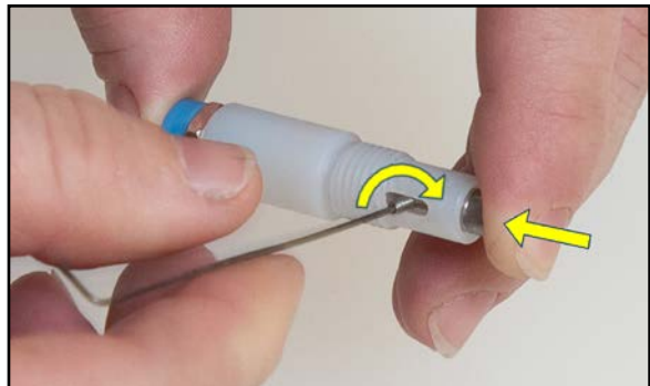
Figure 3-5. Installation of New Internal Brush Assembly (Left) and Set Screw (Right).
