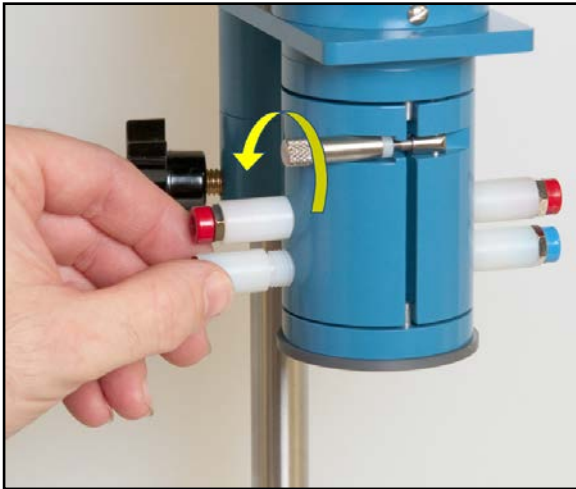
Figure 4-1. Removal of Old Brush Assembly by Turning (Left) and Pulling Out (Right).
